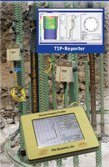
Shape, quality, cage alignment and concrete cover of drilled shafts.
