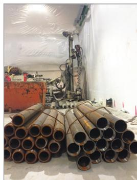
*The Comacchio MC 8 D performing auger drilling and the drill pipes*
