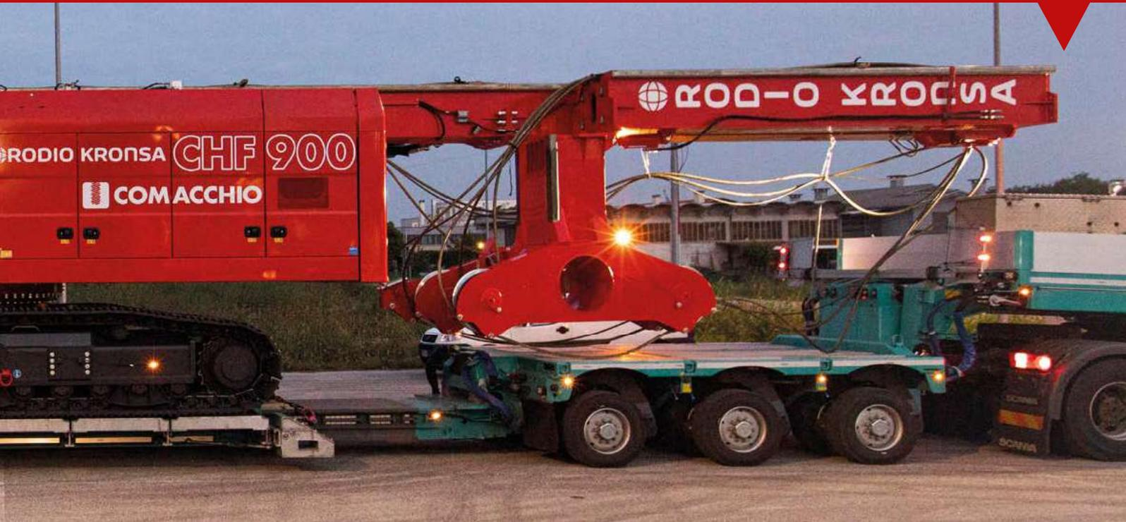
CHF 900 offers an extraction force of 1120kN. An additional 150kN of crowd force on the auger can be provided through an additional pull-down winch on the rotary, available as an option.
