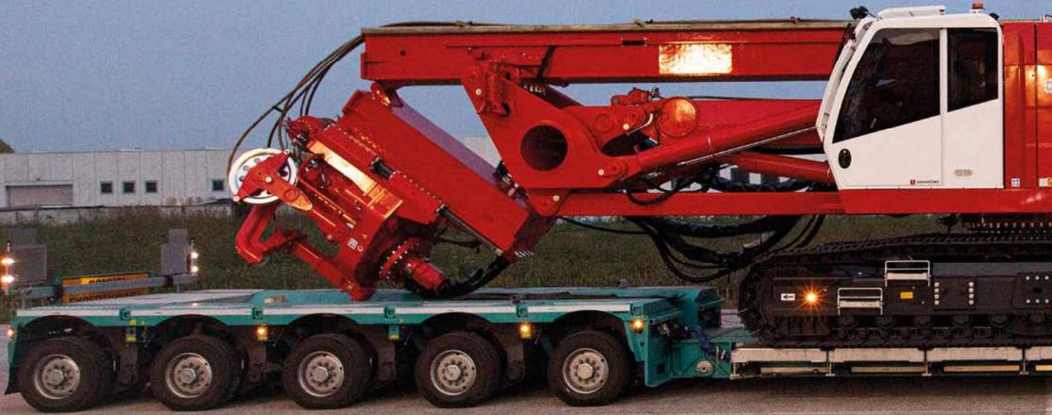
*The weight of the CHF 900 can be reduced to 65.5t in transport configuration*
