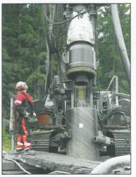
and drill bit. Drill cuttings are then blown up through the centre of the drill bit, RC hammer and drill pipe, and brought out through a 6in (152.4mm) hose pipe for discharge into a container/pond. The equipment supplied to Entreprenørservice by Holte Manufacturing includes a rotary head, 'casing driver', DTH hammer, drill bit and drill pipes.
