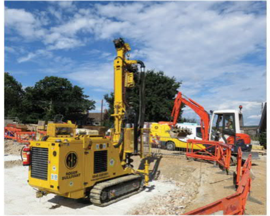
Comacchio's MC 6 F rig, part of the new F-Line series for the mini-piling sector
