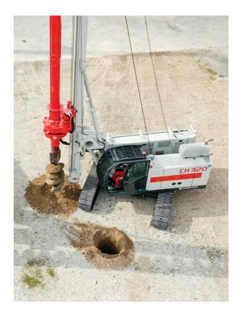
The CH 320 is equipped with a Cummins B4.5 engine, complying with Stage V (EPA Tier 4 Final) emissions standards. Special focus is placed on obtaining the highest energy efficiency. Thanks to the innovative HPE (High Power Efficiency) system, the power supplied to the pumps is electronically controlled in order to
