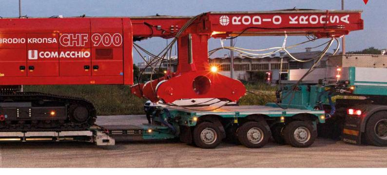
CHF 900 offers an extraction force of 1120kN. An additional 150kN of crowd force on the auger can be provided through an additional pull-down winch on the rotary, available as an option.
