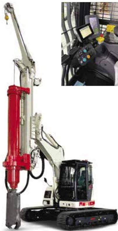
The concept of the new Comacchio CH 150 is based on the use of an excavator base carrier (in the 8-10 tons weight class) equipped with a modular drilling mast and a multipurpose rotary head
