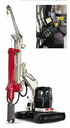
The concept of the new Comacchio CH 150 is based on the use of an excavator base carrier (in the 8-10 tons weight class) equipped with a modular drilling mast and a multipurpose rotary head
