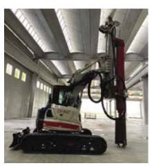
With 2320 mm in width and 3075 mm in length, the CH 150 has an operating and transport weight of 15000 kg and is currently the smallest model in the CH series of Comacchio piling machines
