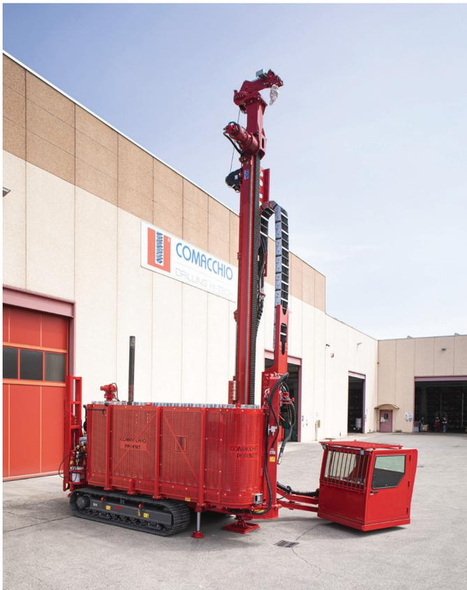
**The CX 2520 grade control rig featuring Comacchio's patented rod carousel and automatic feed system**
