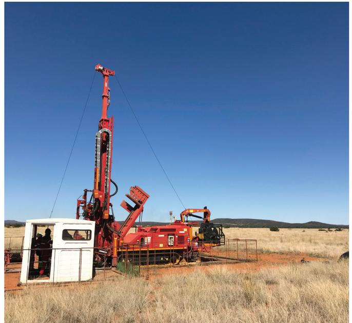
**The Comacchio CX 2030 performing diamond drilling for greenfield exploration with hands free rod handling system**
