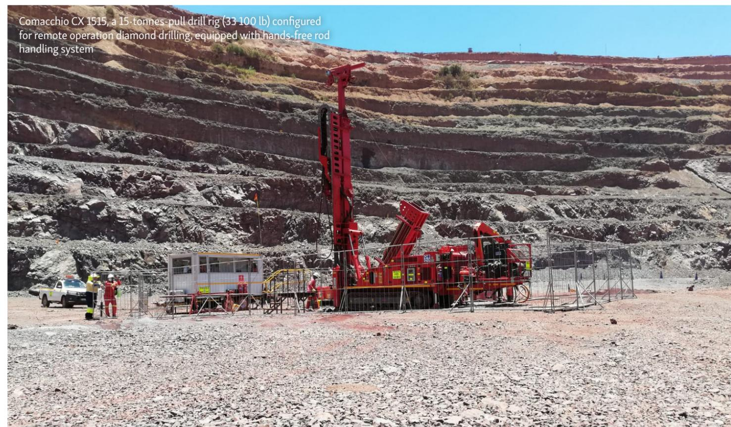
Comacchio CX 1515, a 15-tonnes-pull drill rig (33 100 lb) configured for remote operation diamond drilling, equipped with hands-free rod handling system
